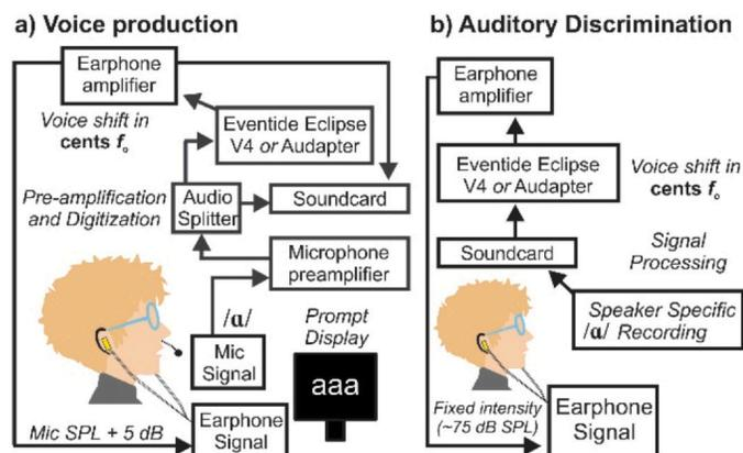
**FIGURE 1.** Experimental setup for shifts in auditory feedback of fundamental frequency ( $f_0$ ). Voice production tasks (a) were calibrated such that auditory feedback was administered 5 dB above the microphone (mic) sound pressure level (SPL). The auditory discrimination task (b) was calibrated such that shifts in voice  $f_0$  were played back at approximately 75 dB SPL.
